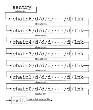
Figure 6: Malicious directory structure to force the victim to sleep on I/O with extremely high probability and hence enable the attacker to win a single race. We call this structure a *maze*. We place an arrow between a symbolic link and the target it references in a dotted box.
