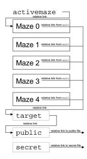
Figure 9: Malicious directory structure for attacking the randomized k-Race defense. The exit links in each maze point to the symbolic link target and the attacker points target to the public or protected file depending on the victim's current system call.
