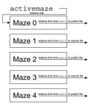
Figure 8: Malicious directory structure to attack the k-Race defense using the maze structure from Figure 6. This construction is particularly effective when k is large.
