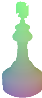
Fig. 3. A typical position map. This is a linearly scaled and clamped high dynamic range image. The red, green, and blue color channels represent x , y , and z world coordinates, respectively.
