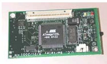
Photo 1. The MICA processor and radio board includes an Atmel chip, which serves as the processor and runs the TinyOS. The board's 51-pin connector interfaces with the sensor boards. On the back side of the processor/radio board is a second 51-pin connector and the radio.
