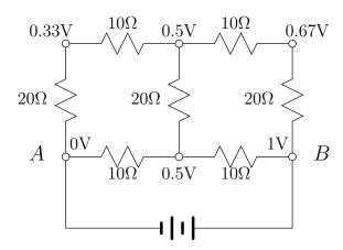
7. Consider a simple resistor grid and a battery, such as in the diagram below:
