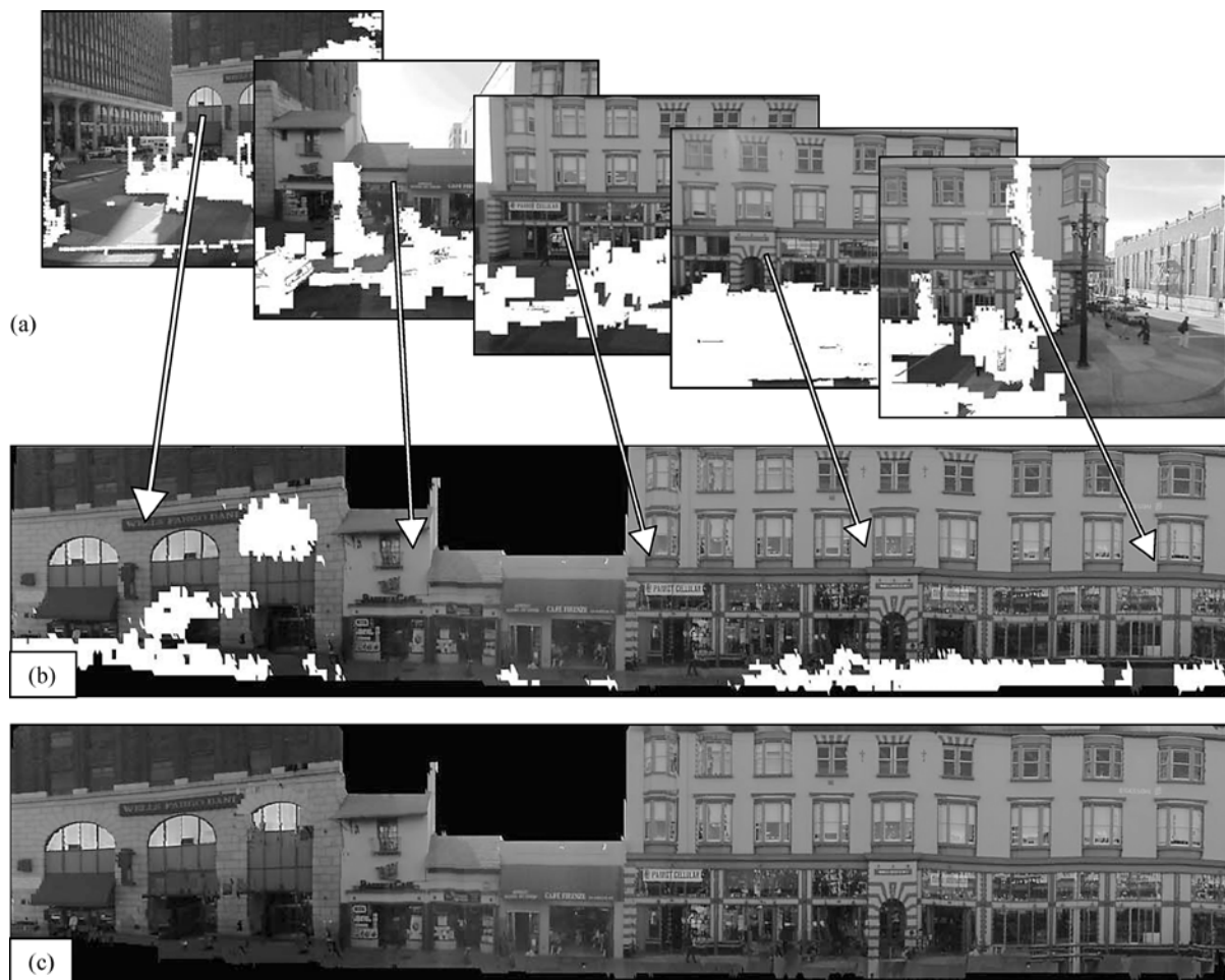
Figure 22. (a) Images obtained after foreground segmentation are combined to create a texture atlas. In this illustration only five images were shown, whereas in this particular example 58 images were combined to create the texture atlas. (b) Atlas with texture holes for the facade portions that were not visible in any image. (c) Artificial texture is synthesized in the texture holes to result in a filled in atlas that is finally used for texturing the background mesh.
