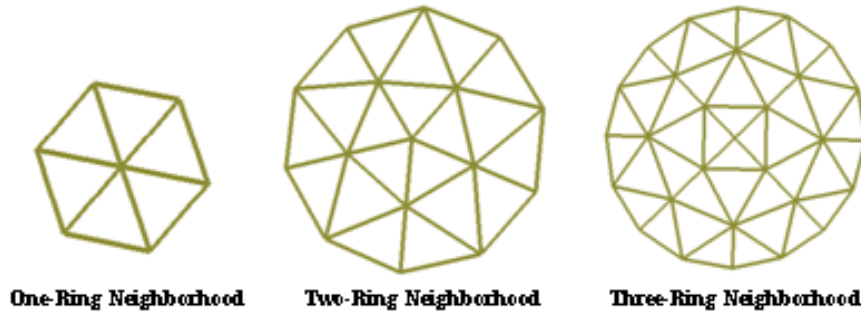
Fig. 1. Sample Test Case Meshes. Left: 1-Ring Neighborhood (valence=6), Middle: 2-Ring Neighborhood (valence=5), Right: 3-Ring Neighborhood (valence=4)
