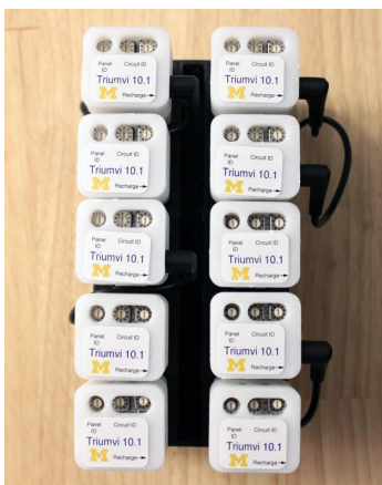
Figure 9.2: Triumvis charging before configuration. The Triumvi storage tray can charge up to ten Triumvis, and it is also a convenient jig for setting the panel and circuit knobs before deploying inside of a panel.
