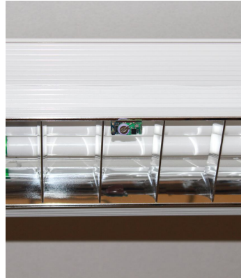
Figure 7.6: Light based occupancy sensor. The energy-harvesting sensor detects state changes in the measured light by detecting when the sensor transitions between different harvesting rates. For example, in a room with only a single source of light, the sensor can detect when the light turns on by observing when the sensor transitions from not harvesting to harvesting. With more ambient light in the room this transition may not be as stark, but there will still be a detectable change in harvesting rate. Timestamping to determine the rate of harvesting is done with a real-time clock.
