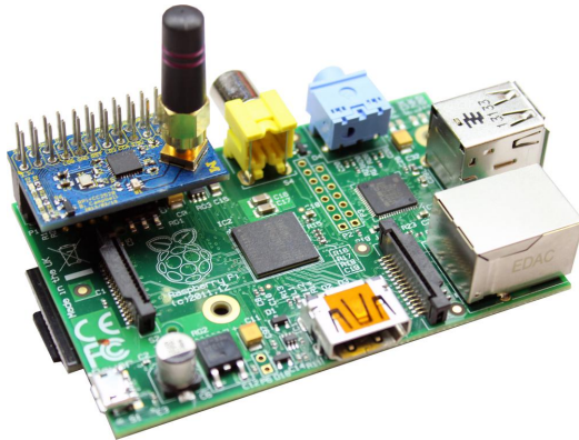
Figure 4.3: RPi Gateway. The gateway is an IEEE 802.15.4 packet receiver shield based on the TI CC2520 radio paired with a Raspberry Pi mini-computer.
