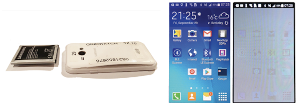
(a) Two swollen batteries.
