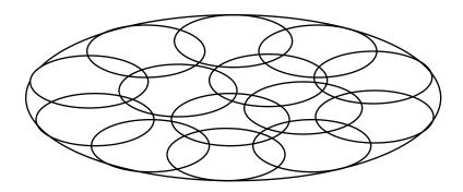
Macrocells for fast movers Microcells for slow movers Estimate speed via doppler frequency Direction-based algorithms
