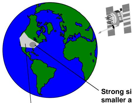
36 MHz transponder: One color TV channel OR 1200 voice channels OR 50 Mbps data rate
