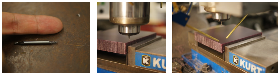
Figure 12: (a) 1/16 diameter tool. (b) Origin-coordinate setting.
