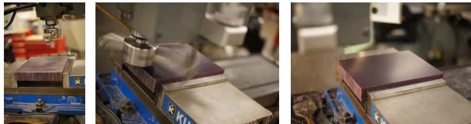
Figure 11: Surface refining process.
