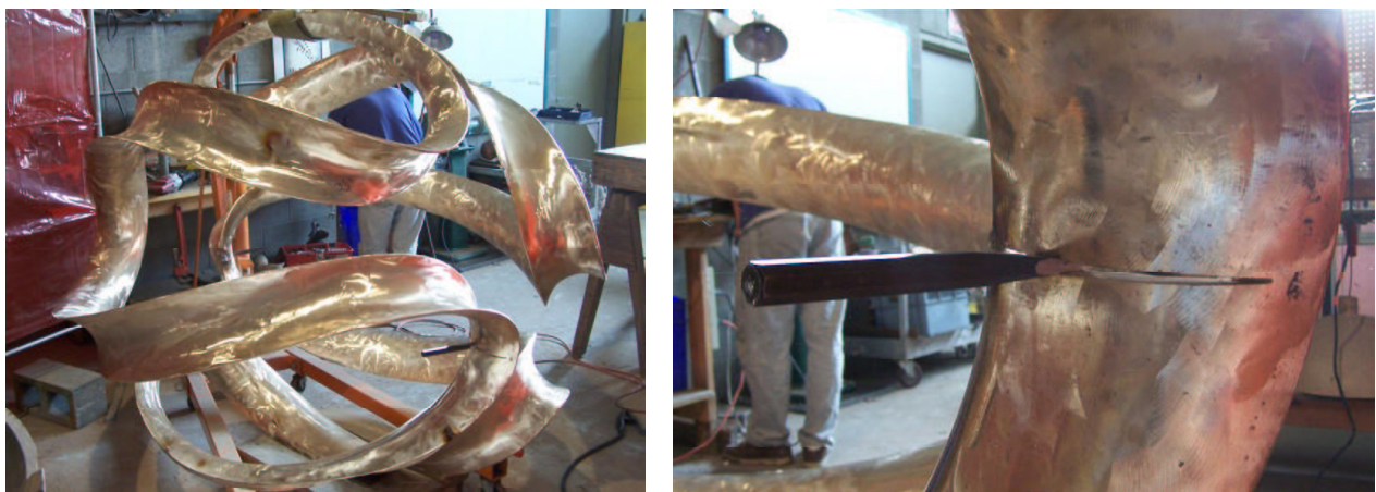
Figure 11: (a) Adjusting the overall shape (b) by cutting the ribbon partly and infilling more material.
