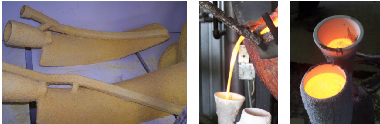
Figure 9: (a) Ceramic shell around wax copies; (b) casting process; (c) cooling bronze in the risers.
