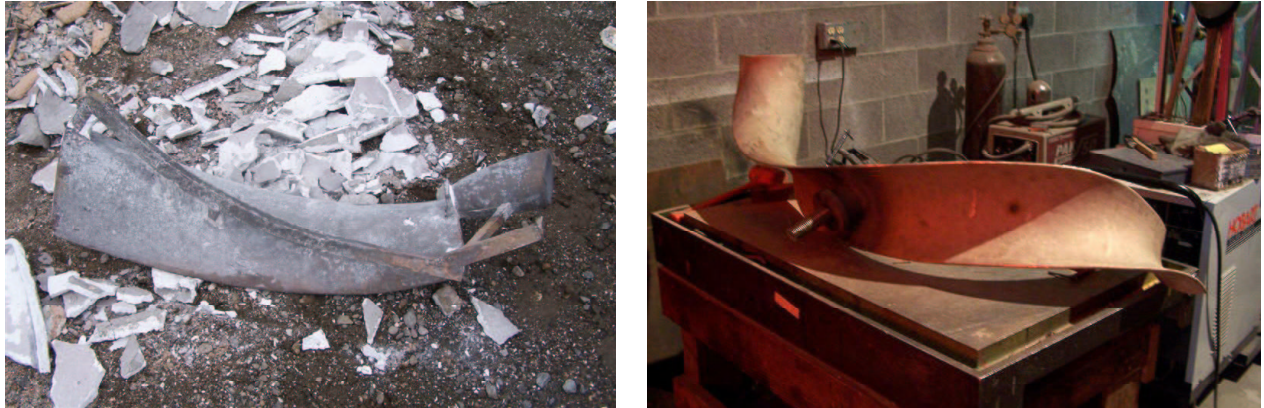
Figure 10: (a) A raw cast piece after ceramic shell has been removed; (b) two of the cast pieces welded together.
