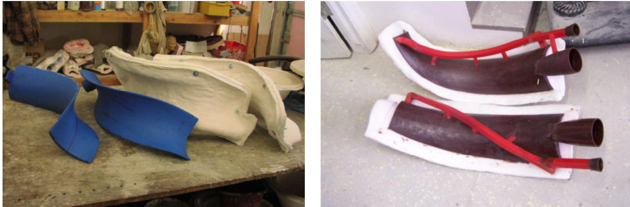
Figure 8: (a) Two sub-segments of the partitioned U-shaped master patterns and their molds; (b) two wax copies of such sub-segments with sprues and risers.
