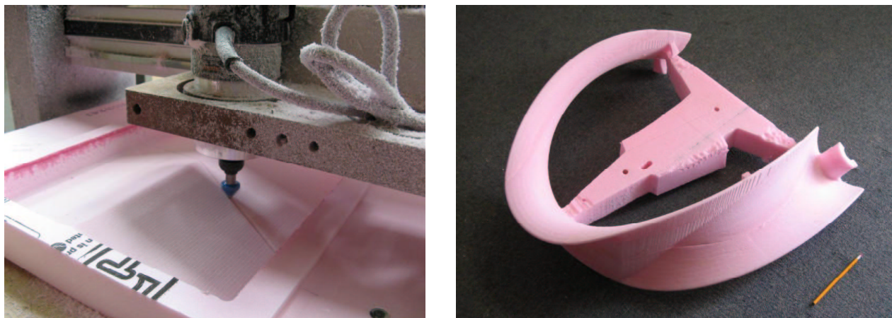
Figure 7: (a) The milling machine used to produce the master patterns; (b) the smaller U-shaped master segment obtained by CNC milling (Photos supplied by Joe Valasek at heartwoodcarving.com).
