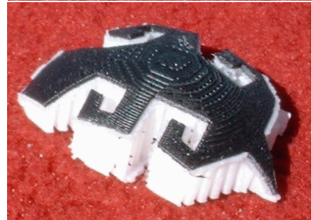
Plate 2. Tiles fresh out of FDM machine.
