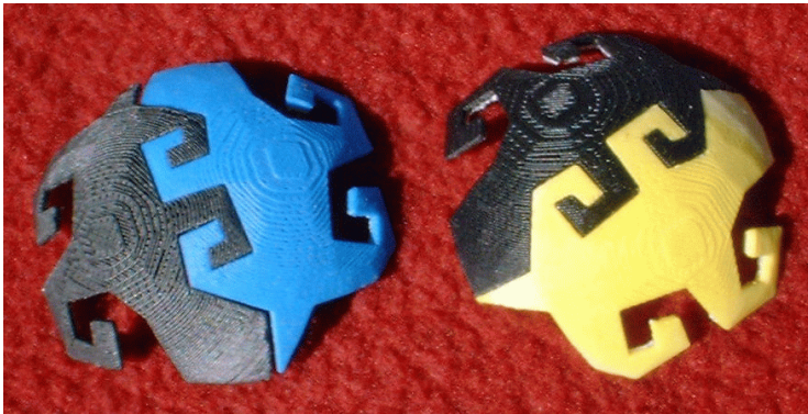
Plate 3. Tiles freed from their support and joined in interlocking pairs.
