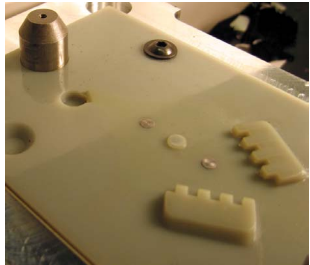
Figure 9 - Mold core after shearing of core pin
