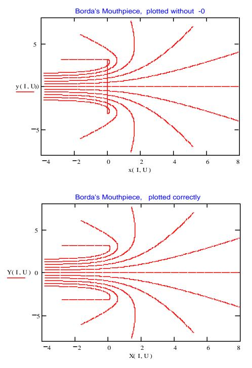
This plot shows the streamlines of a flow of an Ideal Fluid under high pressure escaping to the left through a channel with straight horizontal sides. Inside the channel, the flow's boundary is free, not touching the channel walls. Without -0, the flow along the outside of the lower channel wall is misplotted across the inner mouth of the channel and, though it does not show above, also as a short segment in the upper wall at its inside end. W. Kahan
