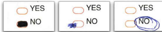
Figure 4.2. Three real-life examples of “No” votes: a correctly classified filled voting target (left), a marginal mark (center), and a mark that was incorrectly classified as an empty voting target because there is little ink inside the voting target itself (right). The latter two cases are examples of potential mark-sensing failures of an optical scan system.
