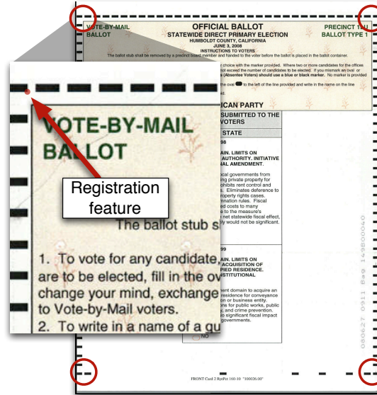
Figure 4.14. To precisely register the ballot images in our set, we first locate the innermost corners of the four outermost hash marks. Given the location of these four points we compute an affine transformation that best maps these four points to corresponding locations in a known coordinate system.
