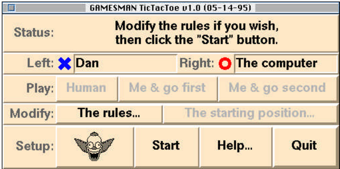
Figure 10.1: The main GAMESMAN interface control window with the Tic-Tac-Toe module loaded in. The play buttons are disabled because the user has not solved the game by clicking on the “Start” button. The “Modify the starting position” button is also disabled because this module does not yet allow for the starting position (in this case, the familiar blank board) to be modified.
