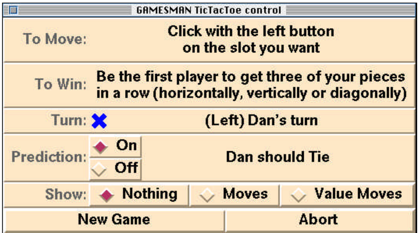
Figure 10.4: The GAMESMAN Tic-Tac-Toe control window. This window tells the user how to move and win in this game, whose turn it is, its prediction of the outcome of the game, and allows the user to augment the game board with a visual display of the available moves, possibly color-coded by value. It also allows the user to restart this game (the "New Game") button and abort the game altogether.
