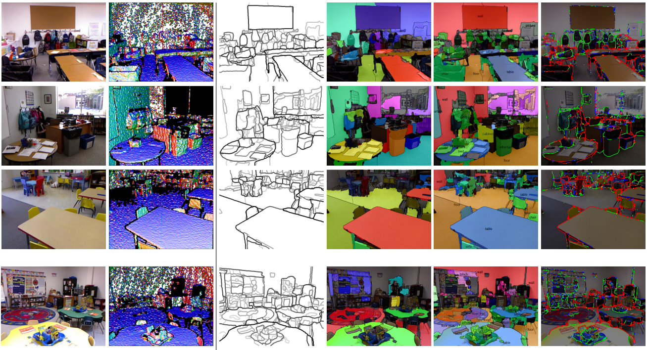
(a) Color Image (b) Depth (c) Contours (d) Amodal Completion (e) Semantic Segmentation (f) Contour Classification
