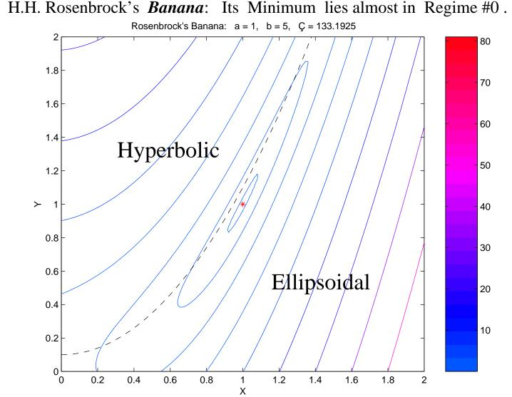
The black parabola, separating hyperbolic from ellipsoidal curvatures, runs so near the Minimum \* that iterates converging to it often straddle the parabola.
