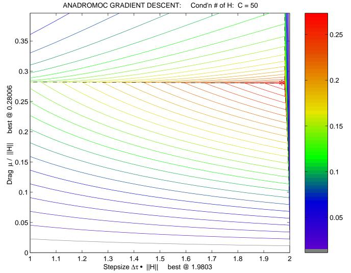
Sub-optimal step-sizes  $\Delta \tau$  and drag  $\mu$  are tolerated well; but the Rate plummets if  $\mu$  is slightly too big.  $\Delta \tau$  slightly too big causes divergence.
