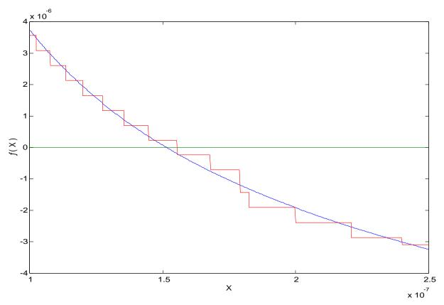
This staircase graph is typical, though the sizes of horizontal steps and vertical risers are often far more diverse. Were roundoff random or biased, the graph of f would appear ragged or shifted, and its zeros  $_k$  would need a trickier program and noticeably longer to be computed "at least about as accurately as the data and the arithmetic's precision deserve". Still, this much accuracy may be achievable only at the cost of several concluding iterations of *Binary Chop*, — too slow.
