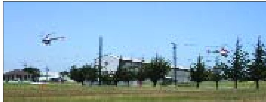
▲ Stills of UAV autonomous collision avoidance experiments (before and after the potential mid-air collision).
