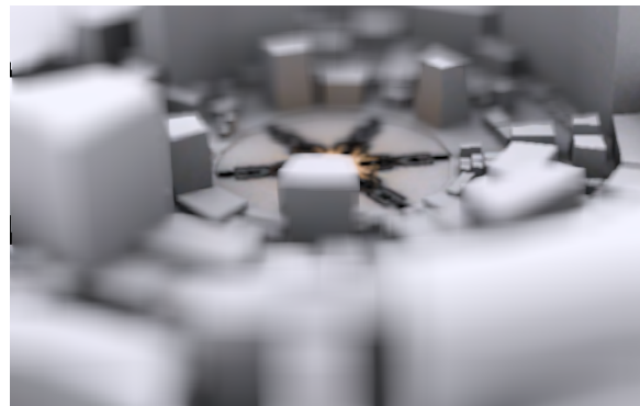
Figure 7: A complex scene, without layers, blurred using rectangle spreading. Depth discontinuity artifacts are reduced. (This 3D model is provided by the Microsoft DirectX 10 SDK.)
