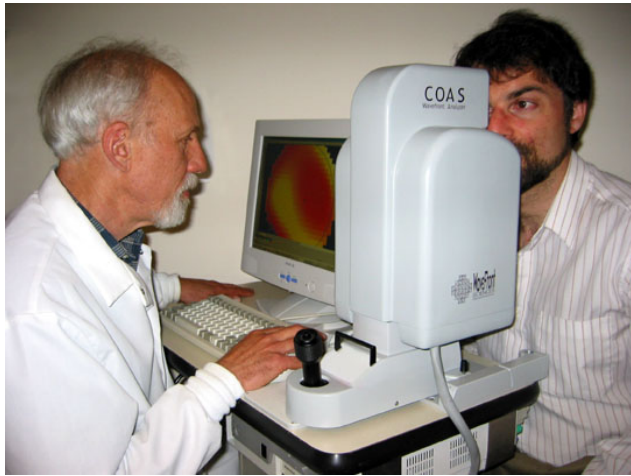
Figure 3: Measuring the specific vision characteristics of a subject using a Shack-Hartmann wavefront aberrometry device.
