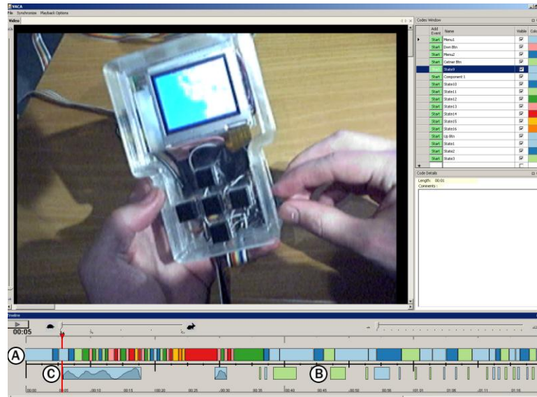
Figure 6.3: The video recording interface in test mode. A: Active states at any point in time are encoded in a timeline view. B: Discrete input events show up as instantaneous events or press/release pairs. C: Continuous input data is visualized in-situ as a small graph in the timeline.
