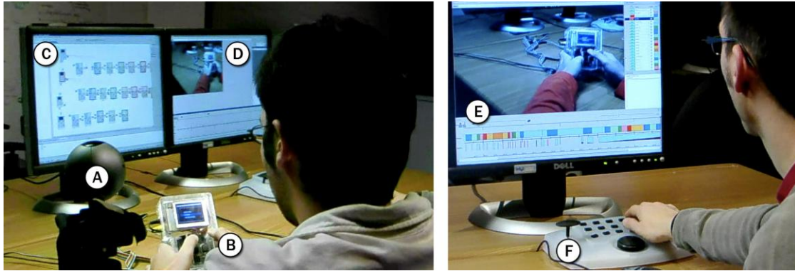
Figure 6.2: Testing a prototype built with d.tools: A camera (A) is aimed at the tester and the physical prototype (B), which is driven by a storyboard (C) in d.tools. Live video of the test is recorded in the video editor (D) and annotated with events and state changes (E). Designers can add additional events to the record with a control console (F).
