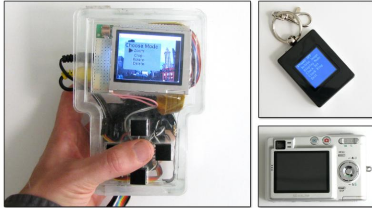
Figure 6.22: Participants were given a prototype device with a color display and button input. They were asked to revise designs for a keychain display and a digital camera, both running on the provided device.
