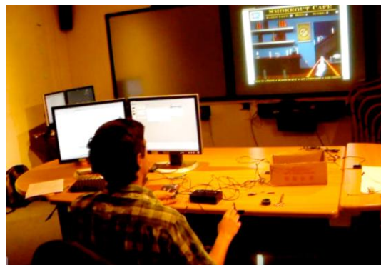
Figure 1.4: This evaluation participant used Exemplar to control 2D aiming in a game with an accelerometer, and shooting with the flick of a bend sensor.
