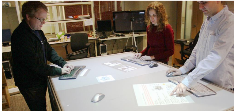
Figure 7.2: The Pictionaire table supports co-located design team work through multi-touch, multi-device input and overhead image capture.
