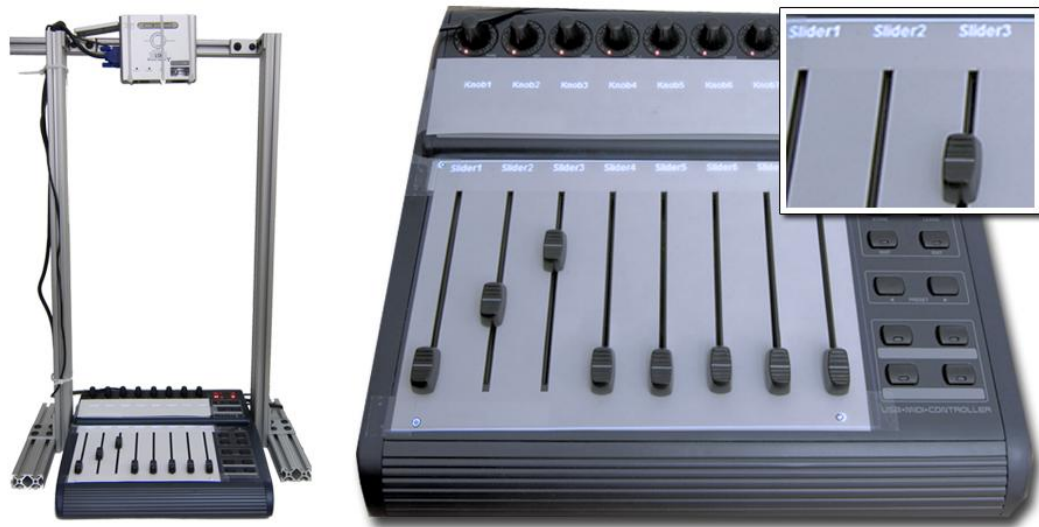
Figure 5.13: An external controller enables rapid surveying of multidimensional spaces. Variables names are projected on top of assigned controls to facilitate mapping.
