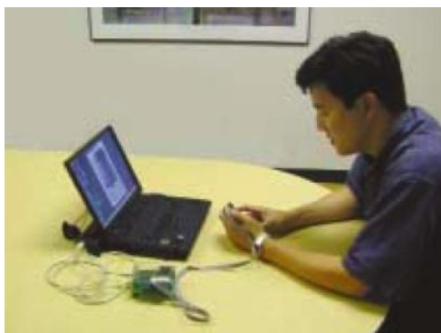
Figure 3.2: Pering’s “Buck” for testing PDA applications: PDA hardware is connected to a laptop using a custom hardware interface. Application output is shown on the laptop screen.
