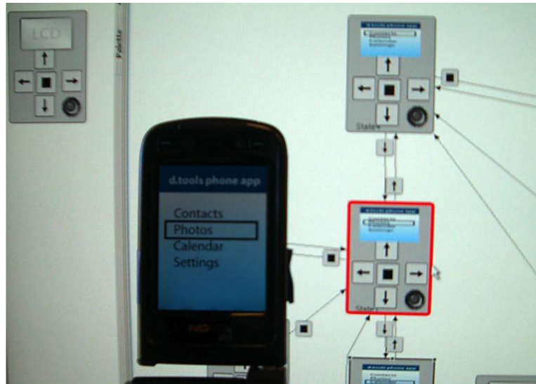
Figure 4.12: A d.tools mobile prototype on a Nokia N93 smart phone, with the storyboard logic of the prototype in the background.
