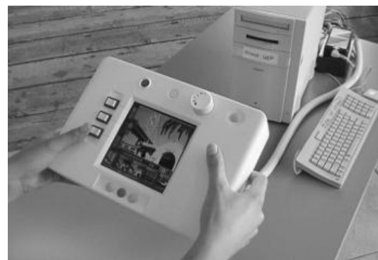
Figure 3.3: IDEO interaction prototype for a digital camera UI. The handheld prototype is driven by the desktop computer in the background.
