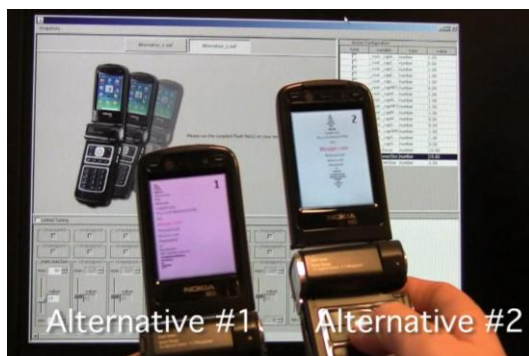
Figure 1.5: Side-by-side execution in Juxtapose enables rapid comparison of alternatives.
