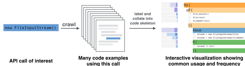
Figure 1. EXAMPLERE takes a focal API call that a programmer is interested in, locates uses of that API call in a large corpus of mined code examples, and then produces an interactive visualization that lets programmers explore common usage patterns of that API across the corpus.
