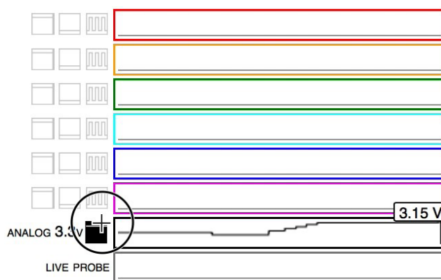
Figure 6: Scope Interface. The first six rows show digital signals over time; To the left of the digital scopes are options to inject signals (HIGH, LOW) or a 1hz square wave. The black "ANALOG" row can either show or inject analog voltages (here, an analog voltage of 3.3 is being injected). The last row reflects the live probe measurements over time.
