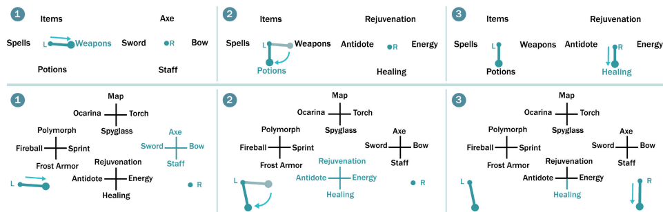
Fig. 17. Top: Hierarchical Display—The left hand explores the parent menu items by dragging through menu items, and the child menu items continuously update for the right hand. Bottom: Full-Breadth Display—The entire menu space is displayed, and the left hand chooses the four-item cluster, while the right hand chooses the item within a cluster.
