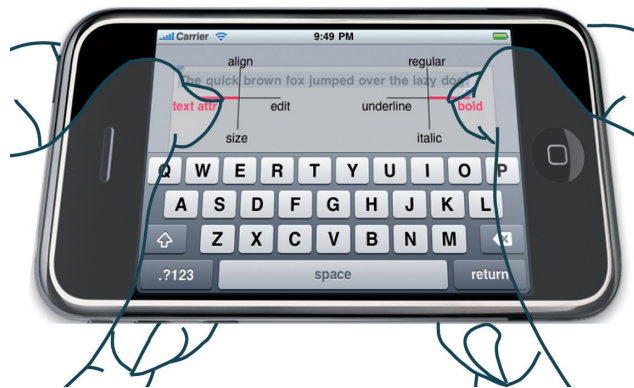
Fig. 1. Using a two-handed ordered marking menu the left thumb strokes to select “Text Attributes” and then the right thumb selects “Bold” to modify the sentence. With a two-handed simultaneous marking menu, users draw both strokes at the same time.
