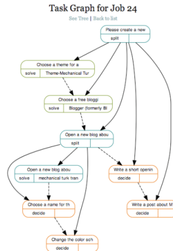
Figure 4: Turkomatic includes a real-time visualization and editing interface. Each node represents a task generated by a crowd worker; the color indicates whether it has been solved or not. Requesters can click to modify either the plan or the solutions to any step to eliminate worker errors or search for alternate solutions.
