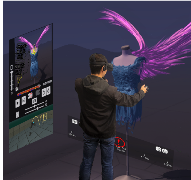
Figure 1: An overview of our VR-embedded tutorial system. Our video widgets (on the left and below the user) can be rendered directly inside the user's active VR painting application (TiltBrush in this example). The user can access useful tutorial content while painting and can interact with the video widgets to explore and learn at their own pace.
