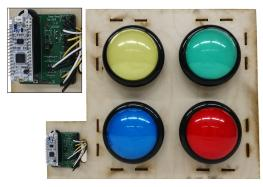
Figure 11. The Simon PCB (with detail view) and connected buttons.
