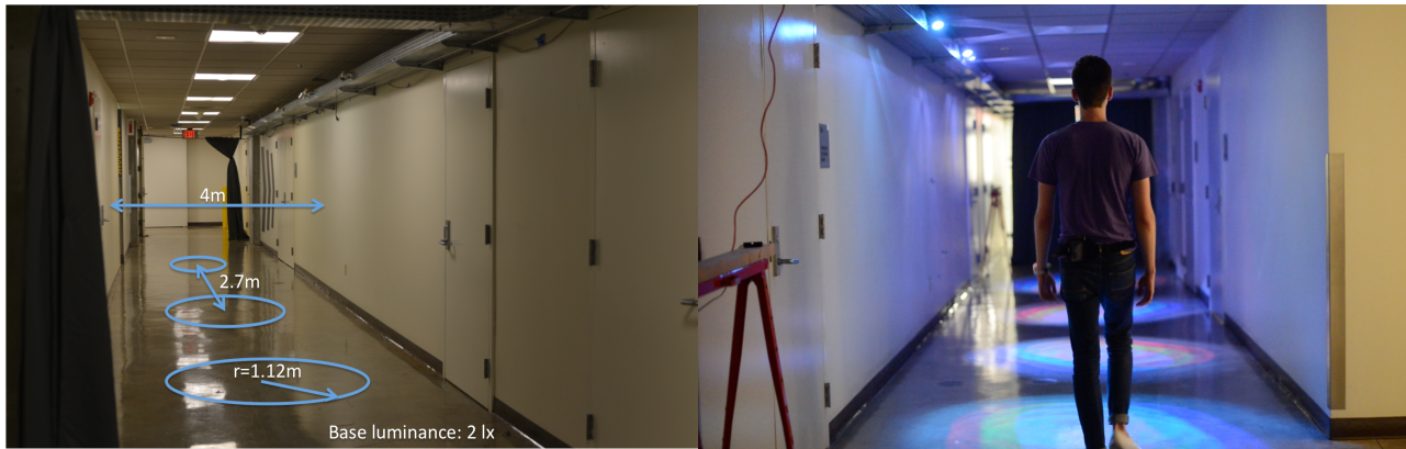
Figure 2. Experimental setup a) metrics: light radius = 1.12m, distance between lights = 2.7m, hallway width = 4m, hallway length = 30ft, base luminance with lights off = 2 lux. Note: low illumination not displayed in this image; b) User walking with all lights on. Max luminance per light = 40 lux. Note: Image captured with high sensitivity camera, appears to be brighter than reality.
