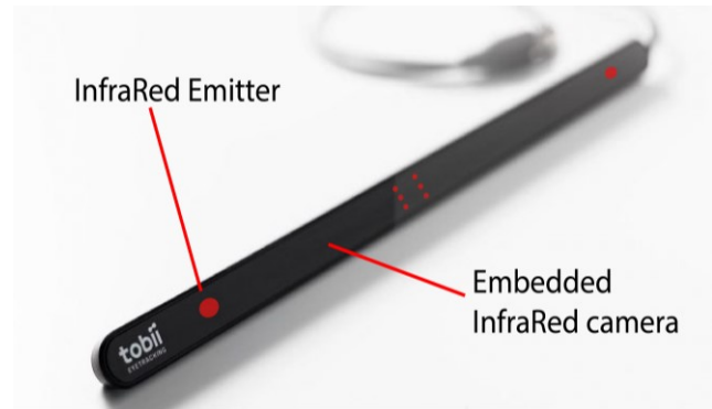
Figure 2. Tobii Eye Tracker 4C sensor before mounting to a computer.
