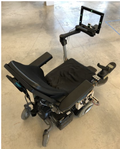
Figure 12. The wheelchair used for this research, with the See-Thru prototype mounted on the left side.
