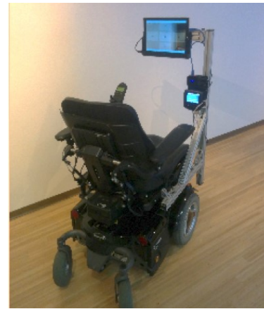
Figure 4. An example of a conventional eye-controlled wheelchair design made by Microsoft Research.
