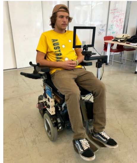
Figure 1. The See-Thru interface mounted onto a power wheelchair.
