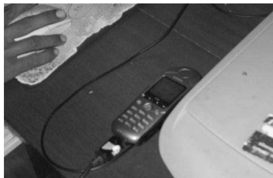
Figure 9: A cellphone-based GPRS modem providing 9.6kbps connectivity to a CIC center in Cambodia.
