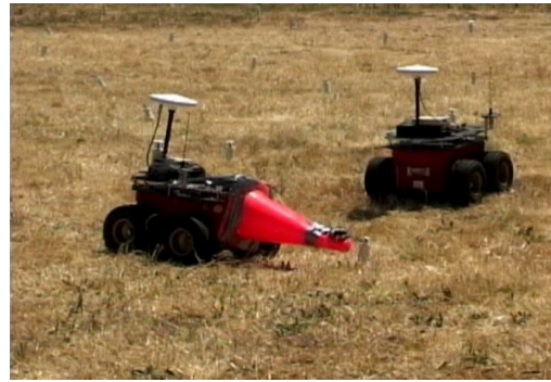
Figure 7: Object tracking applications. left) indoor testbed with 25 nodes, a RC car and a pan/tilt camera. As the remote control car is driven through the sensor field, the network locates the car and send the position to the camera, which visually tracks the vehicle. right) real outdoor deployment with 100 nodes, and two robots. As one robot moves, the network reports its position to the second robot (with the safety cone), which pursues it autonomously.
