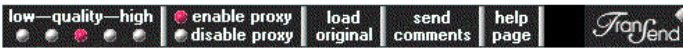
Figure 3: The Java “Dashboard” that is inserted at the top of each page served to the user through the proxy.
