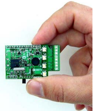
Figure 2. SG-Link™ wireless strain gauge node (MicroStrain, Inc)
