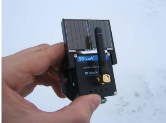
Figure 5. Integrated solar energy harvester and wireless strain sensing node.
