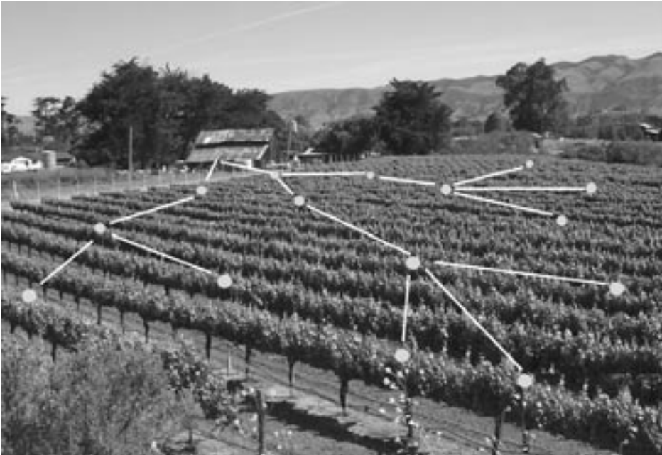
Figure 1. Ad hoc, wireless embedded network for precision agriculture. Sensors detect temperature, light levels, and soil moisture at hundreds of points across a field. The system communicates the data over a multihop network for analysis.
