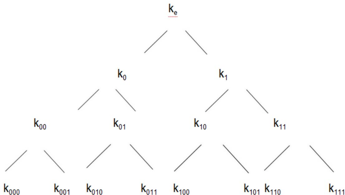
The scheme can be represented as a binary tree, where each leaf is a BluRay player, each node is a key, and the keys are all unrelated to each other. An example is shown above, where in this case there are 8 players. Each player is given all the keys of its direct ancestors up to the root node. For example, the player with  $k_{101}$  will have the keys  $k_{101}$ ,  $k_{10}$ ,  $k_1$ , and  $k_e$ .
