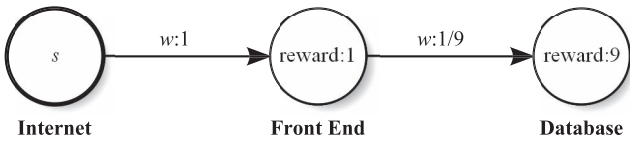
Fig. 2. Attack graph representing a simplified data center network.
