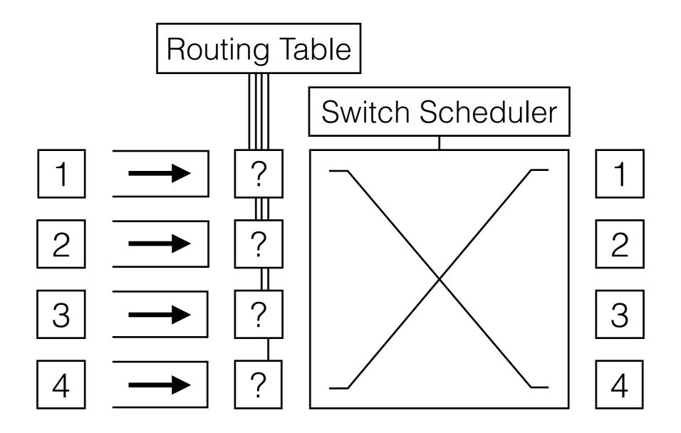
Routing table —> SRAM based CAM
