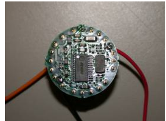
A Mica2Dot mote (radio chip in the middle)
