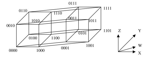
The processors are number with 4-bit binary numbers which represent the X-Y-Z-W coordinates
