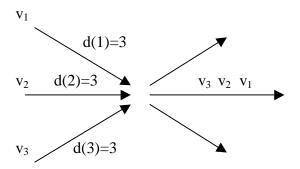
e.g. in the figure above, three packets arrive at the same node and attempt to leave along the same link (we show their destinations as the same which doesn't happen with permutation routing, but what we really mean is that the next node address is the same). If the 3 packets arrive at time step T, the packets are queued, and  $v_1$  leaves in time step T+1,  $v_2$  leaves at T+2, and  $v_3$  leaves at T+3.
