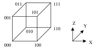
The processors are at the vertices of the cube, and edges represent communication links. Each processor is numbered with a 3-bit binary number. Notice that the processor numbers are also X-Y-Z coordinates of the 3D layout of the cube.
