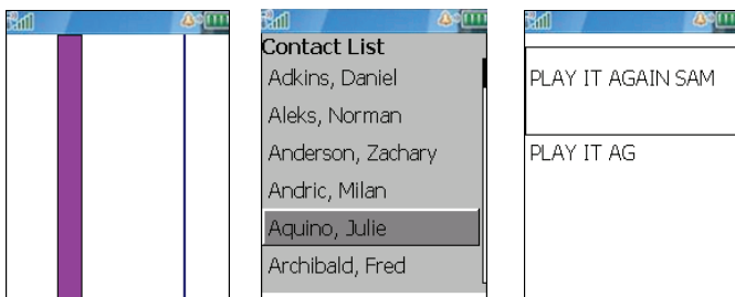
Figure 4: From left to right, screen shots of the target acquisition task, menu selection task and text input task.
