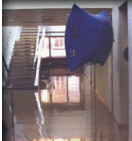
FIGURE 3: A blimp tele-robotic space browser traversing a building
