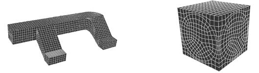
Figure 4. Examples of all-hex meshes generated automatically be the Geode algorithm.
