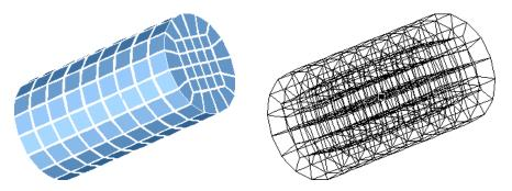
Figure 22: Hexahedral mesh for a cylinder (part of the model in Fig. 20). The cycle elimination scheme first selects parallel cycles corresponding to eight layers, and uses than a double elimination to remove the 16 hexahedra forming a torus on the last layer.
