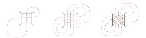
Figure 17: Getting rid of a self-intersecting dual cycle (left): the dual cycle is first duplicated (middle), and then the surface mesh is locally transformed (right).
