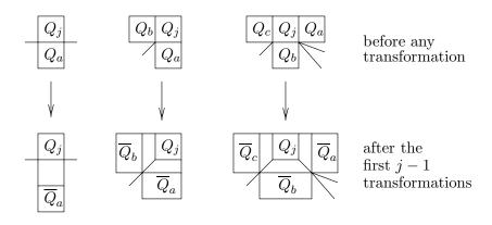
Figure 6: The different cases of local subgraphs before a hexahedron is placed on top of quadrilateral  $Q_j$  ( $Q_a, Q_b$  and  $Q_c$  come before  $Q_j$  in the shelling order). The number of quadrilaterals sharing a corner with  $Q_j$  and lying "between"  $Q_a$ and  $Q_b$  (or "between"  $Q_b$  and  $Q_c$ ) can be an arbitrary non-negative number (including zero!).
