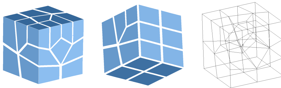
Figure 8: The “doublefold” example (the middle picture is the left cube with the front faces removed so you can see through to the back faces from the inside). The hex complex consists of 17 hexahedra.
