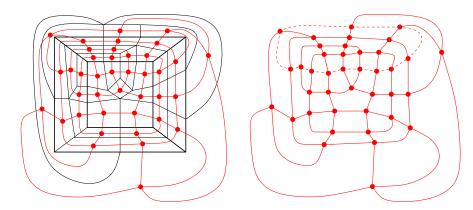
Figure 9: The primal and dual graph of the surface mesh of the "double fold" example, dual nodes are drawn as solid circles (left); the first dual cycle of a perfect elimination scheme is dashed, it encloses 9 dual nodes (right).
