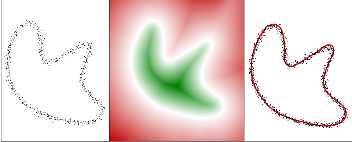
Figure 4.1: (a) A two-dimensional data set with added noise. (b) Cut function defined by the uniform MLS algorithm. (c) Zero set of the cut function.
