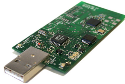
Figure 1: Telos ultra-low power wireless module ("mote") with IEEE 802.15.4 wireless transceiver.
