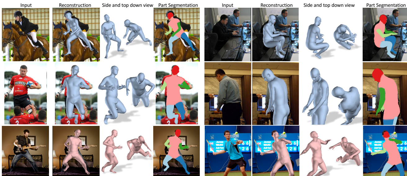
Figure 1: Human Mesh Recovery (HMR): End-to-end adversarial learning of human pose and shape. We describe a real time framework for recovering the 3D joint angles and shape of the body from a single RGB image. The first two rows show results from our model trained with some 2D-to-3D supervision, the bottom row shows results from a model that is trained in a fully weakly-supervised manner without using any paired 2D-to-3D supervision. We infer the full 3D body even in case of occlusions and truncations. Note that we capture head and limb orientations.
